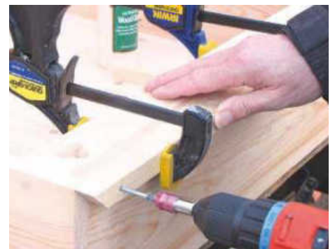
STEP 16. Mitre, glue and screw 20 x 20mm blocks around the top of the carcass to support the coving
